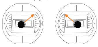
At the same time turn on the remote control and enter the joystick calibration / restore factory status, the remote control will rattle and the power indicator light will flash, first rotate the two joysticks on the remote control up, down, left and right by the maximum range for one full circle, as shown in the following figure,
