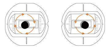
Then flick the joystick to the center position as shown below, finally toggle the car speed switch, sound stops, power indicator stops flashing, joystick calibration / restore factory is complete.
